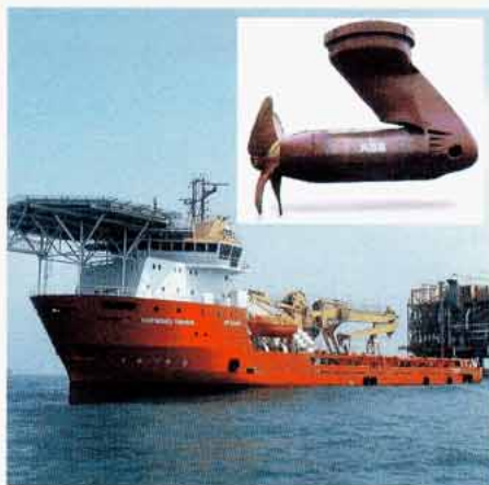
»Normand Rover« built at Aker Yards Søviknes Verft in Norway and her Compact Azipod from ABB
