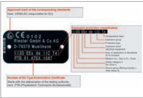
Figure 4. Marking of an explosion-proof device. Test name plate of an AUMA actuator
