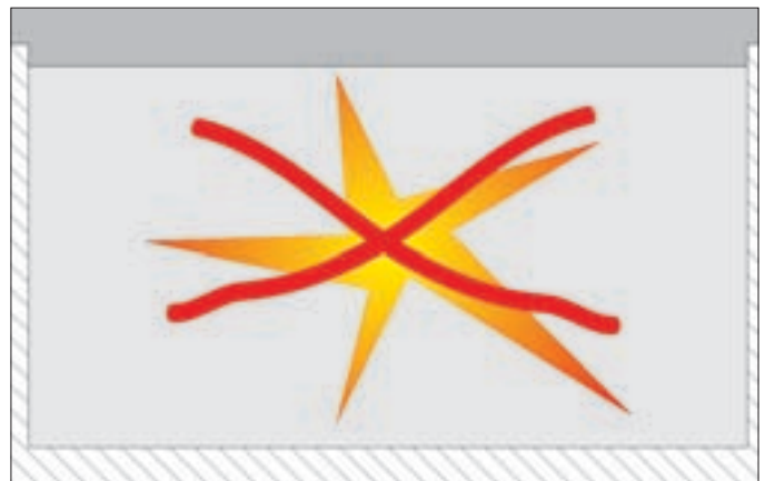
Figure 3. In contrast to the 'Flameproof enclosure' explosions in 'Increased safety' areas are impermissible.
